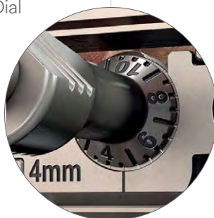
Dial shows an offset position between 4 and 5
